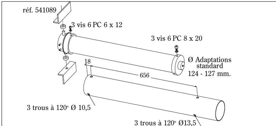
**FIXATION DU MOTEUR DANS LE TUBE**
